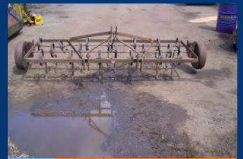
1166513 Kongskilde kkk £ 250, H J Knight & Son, Tel. +44 1243 575333, hjk.eastashling@yahoo.co.uk, Hitch, Spring tines, 3 point linkage mounted spring tine. Depth wheels all tines & points in place.
